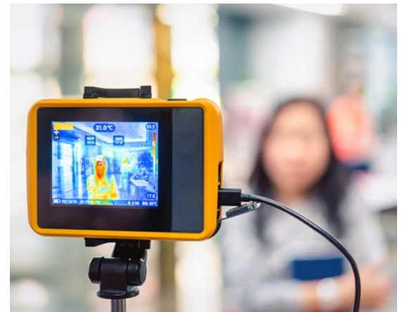
Figure 1. Temperature screening system with a thermal imaging device
