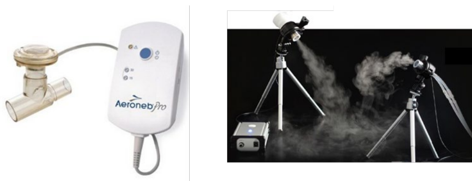
Figure 1. Photographs of possible liquid/particulate simulant release devices. A combination of a nebulizer (left) and a droplet generator (right) would be used to generate small and large droplet size distributions. During the study, release devices may be linked together with small holding chambers and source of compressed air to generate a specific release velocity.
