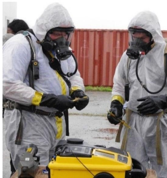
*First responders inject a sample into the Tridion-9 portable gas chromatograph during Urban OpEx 2016*
