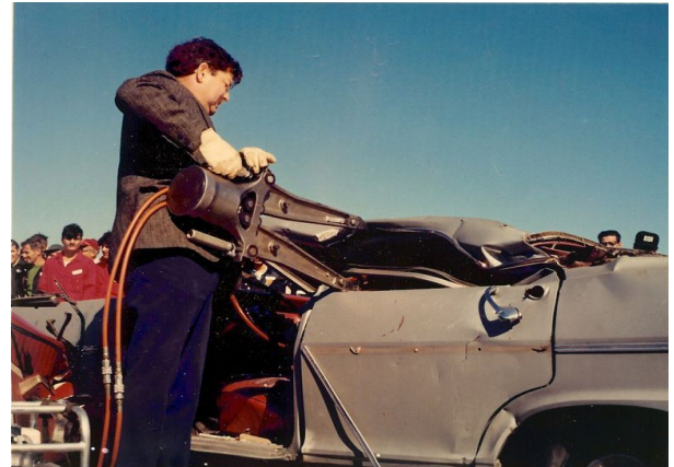
Figure 1. An early version of the Hurst Power Rescue Tool Image credit: Kevin Brick and National Museum of American History
