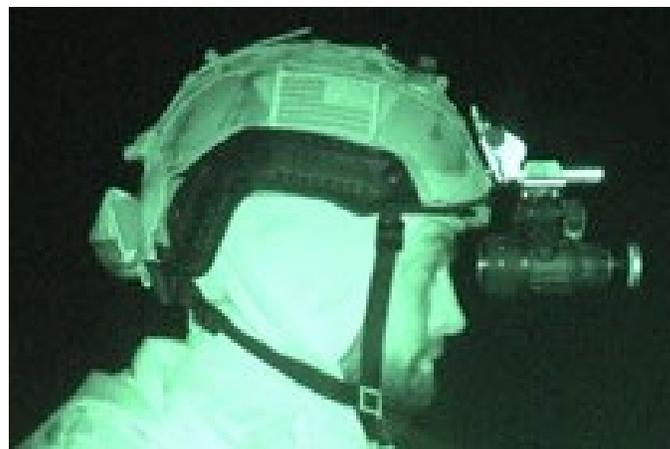
Figure 4. This profile of a helmet-mounted BNVD shows the distance between user and device.
