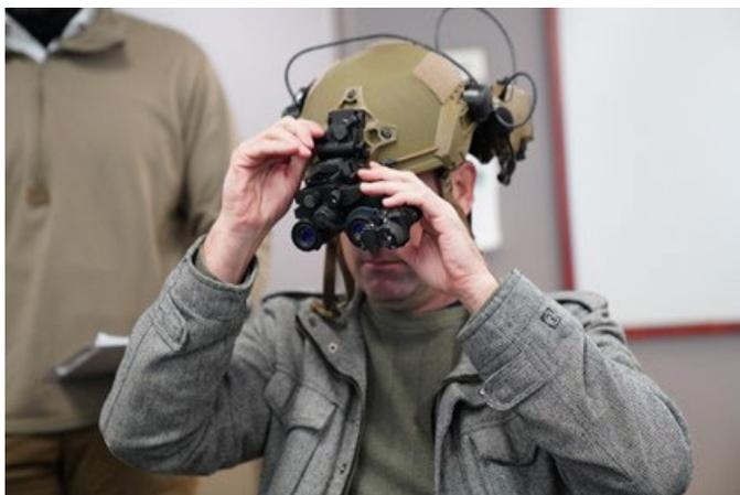
Figure 3. An evaluator wears the PRG Defense NVG-51 with ECOTI thermal accessory.
