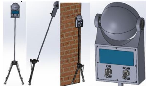
Sample use case: Leaning Tripod/Radar Stick
