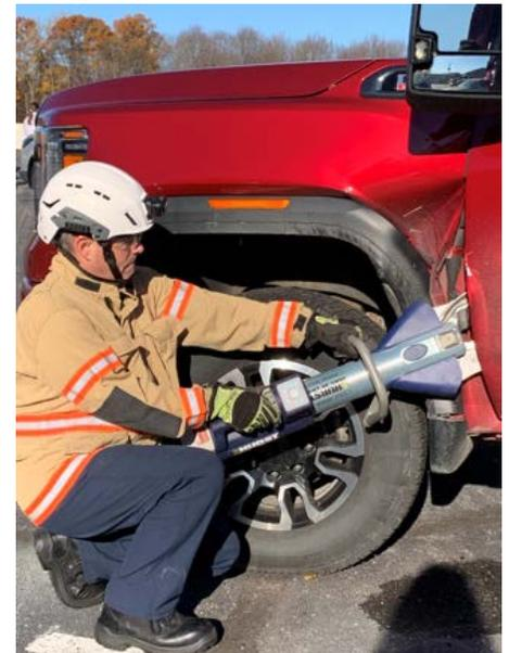
Figure 1. An evaluator uses a HURST S789 E3 cutter on the driver-side door of a truck.
