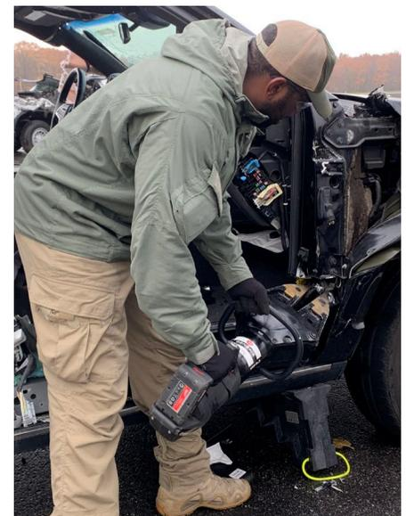
Figure 2. An evaluator uses a Genesis S49-SL3 EForce spreader on the A pillar of a vehicle.
