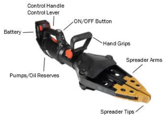
Figure 2-1 Genesis S49-SL3 EFORCE spreading tool with external components labeled
