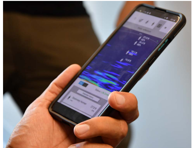
Figure 3-2 Multiple targets detected at range of up to 27 feet
