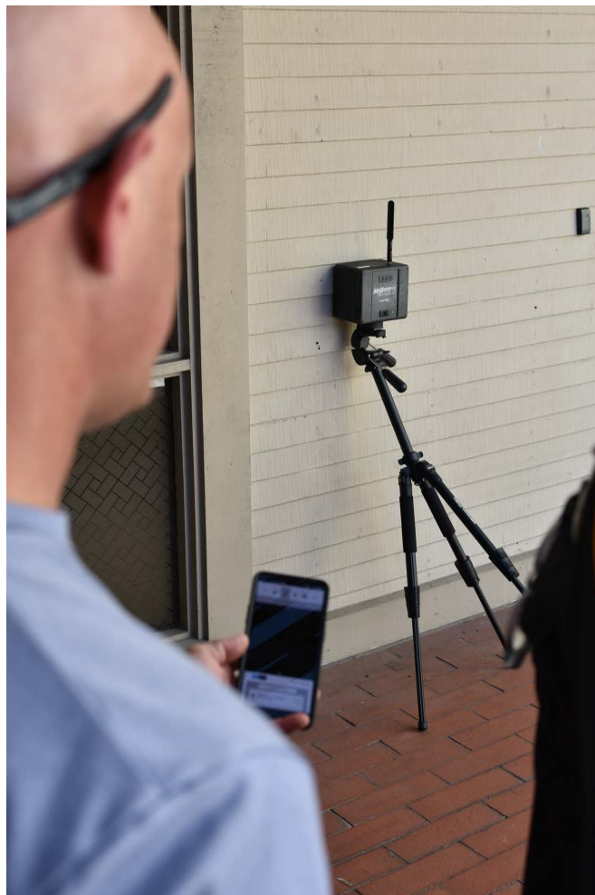
Figure 3-3 Device deployed with tripod against exterior wall
