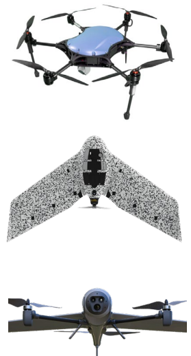
Figure 1. Multirotor (top), fixed wing (center) and hybrid (bottom) are the primary UAS platforms.
