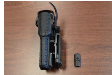
Figure 5-2 Yardarm Holster Aware sensor affixed to the holster and on a desktop
