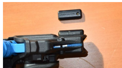
Figure 5-3 Utility Smart Holster sensor affixed to the holster and laying on a desktop
