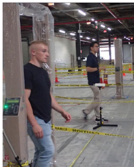
Figure 3-5 Portal monitor walk-beside tests Top—at NUSTL Bottom—at NYC CRC training facility
