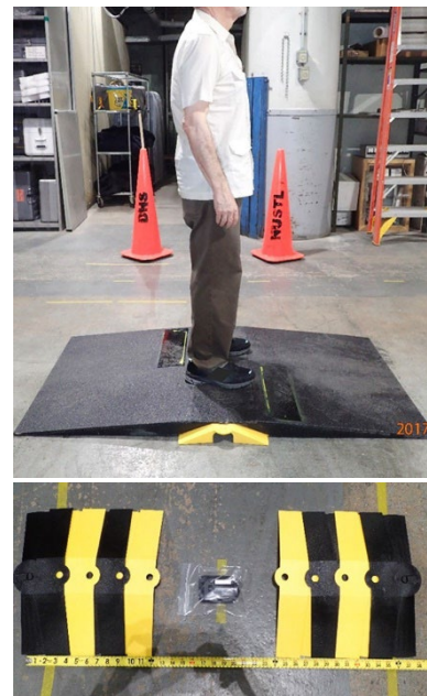
Figure 3-10 Prescreening shoes with a PRD under a ramp Top—client standing on ramp Bottom—PRD between ramp supports
