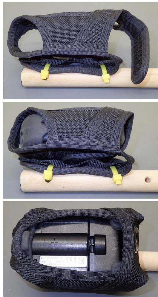
Figure 7-20 Holster method for mounting a PRD on a handle Top—holster attached to handle with zip ties Middle and Bottom—PRD in holster
