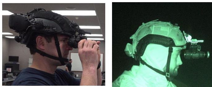
Figure 4-11 Helmet-mounted DTNVS highlighting the gap between the user's eyes and the device
