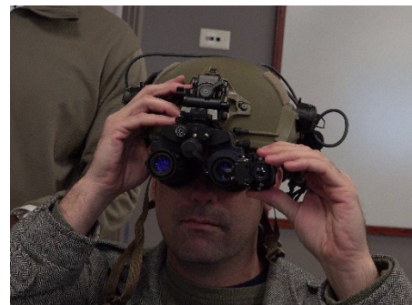
Figure 4-19 Evaluator adjusting the ECOTI affixed to the PRG Defense NVG-51
