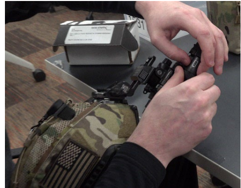
Figure 4-6 An evaluator attaches an ECOTI to the L3Harris BNVD-1531
