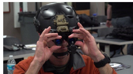
Figure 4-22 Evaluator adjusting the focus on the Nightline RNVG with the ECOTI affixed
