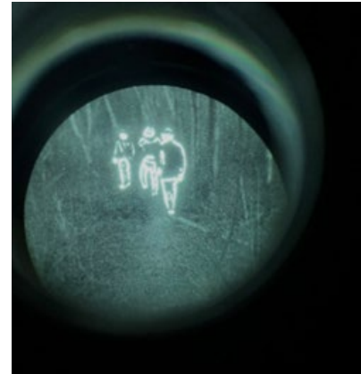
Figure B-4 View through ECOTI in outline mode in a wooded area
