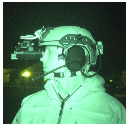
Figure 4-5 This profile view of an evaluator wearing a mounted L3Harris, BNVD-1531 illustrates its fit against the user's face
