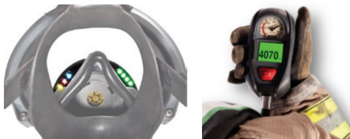
Figure 2. A HUD built into a facepiece (left) uses color-coded LED indicators, while the pressure gauge (shown right) uses both analog pressure displays and digital graphical displays of numeric cylinder pressure, battery status, alarms, and remaining service time.
