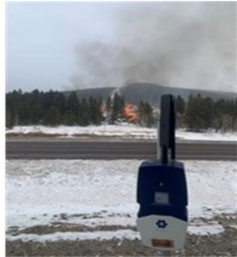
N5 Sensor detects unusual concentrations or spikes in levels of particulates or carbon monoxide to detect wildfire ignition.
