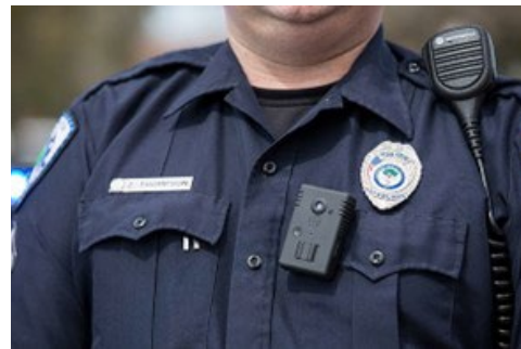
Figure 2-2 BWC attached by a magnetic mount.
