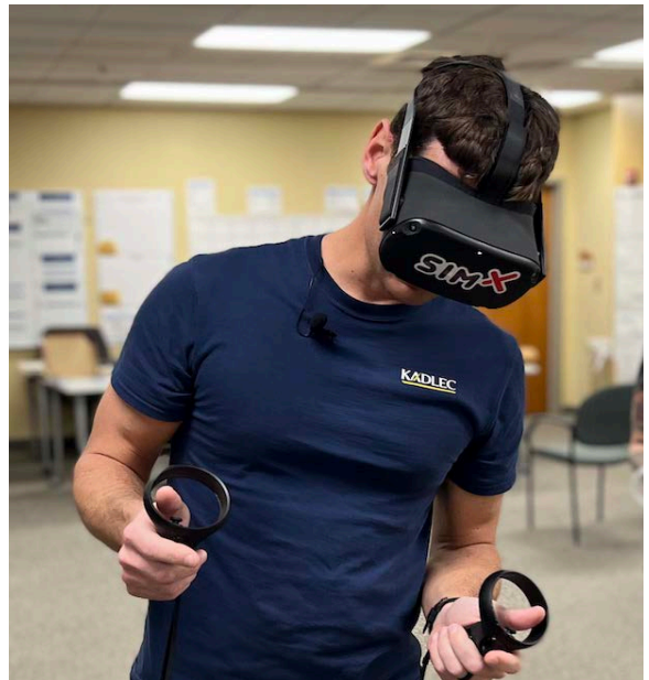
Figure 2-1 Standalone VR HMD with handheld controllers
