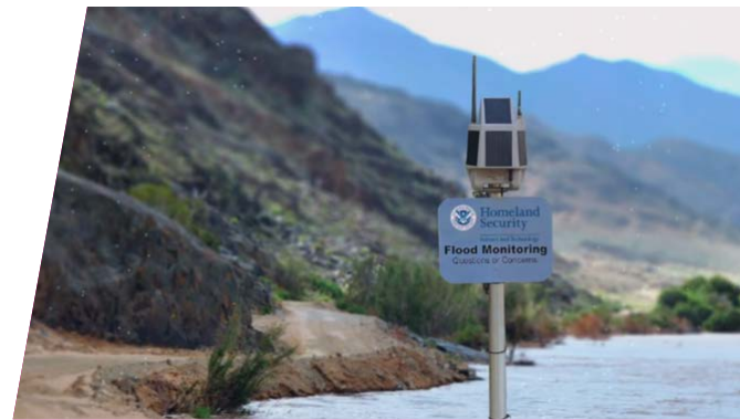
Internet-of-Things flood sensor performing monitoring. Photo: S&T
