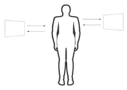
The figure depicts the implementation of a human phantom containing the artificial skin used to test active MMW imaging systems to determine whether the systems are capable of distinguishing between human skin and a threat object.
