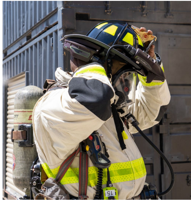
Figure 3-4 Evaluator attempting to adjust helmet fit using the ratchet under C-THRU Navigator hardware
