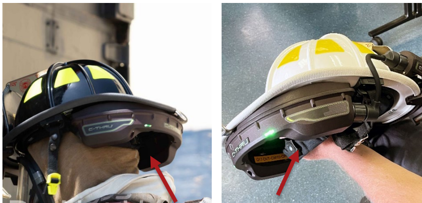
Figure 3-14 Ratchet in relation to C-THRU Navigator hardware while worn (left) and in hand (right)
