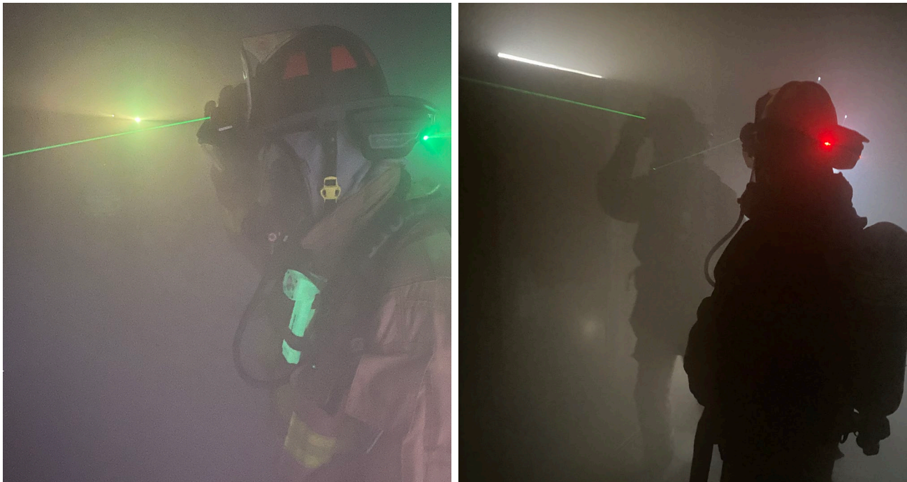
Figure 3-6 Laser in use during operational scenarios and taillight shift from green (left) to red (right) indicating Mayday mode
