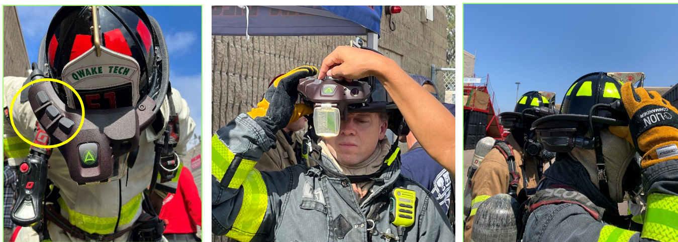
Figure 3-15 Control buttons configuration (left) and view of gloved hand on control buttons from the front (center) and profile (right)
