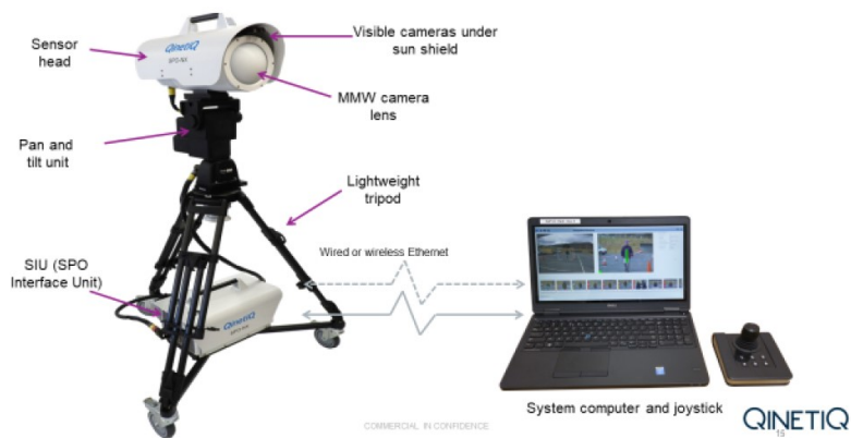
Figure 4-6 Qinetiq SPO-NX system components
