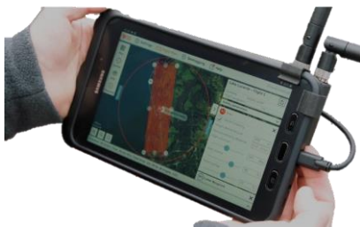
Figure 3-17 WingtraOne Gen II and rugged Samsung Galaxy Tab Active 3 ground control station
