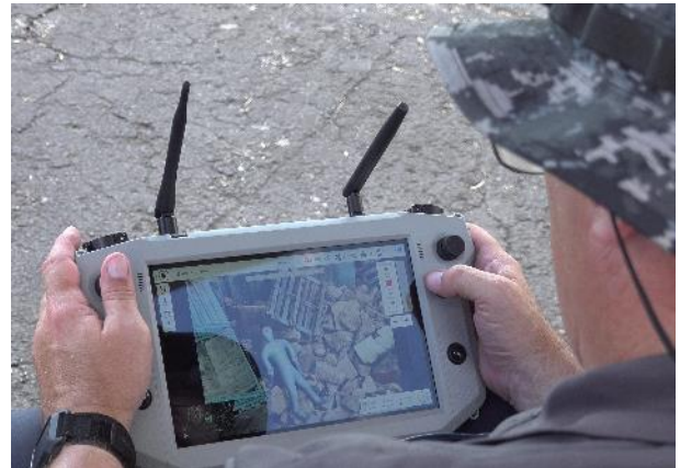
Figure 3-2 Evaluator using the Teal 2 to locate a victim in a rubble pile
