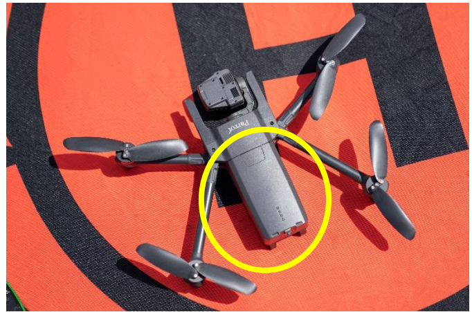
Figure 4-11 Aerial view of the ANAFI USA GOV, with the battery (circled in yellow) attached noted
