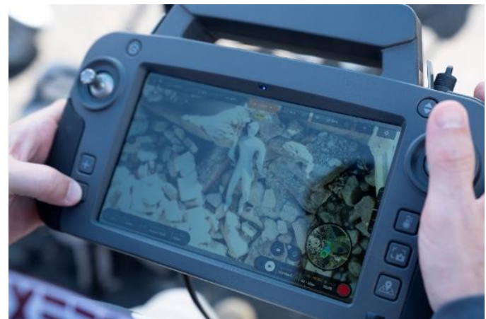
Figure 4-9 Evaluators locating a casualty during daytime operations on the ANAFI USA GOV GCS (Skycontroller 3)
