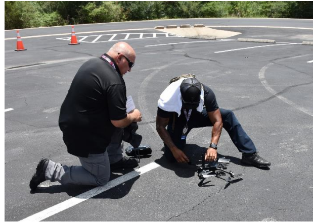
Figure 4-20 Evaluators configuring the and rotors of the Skydio X2D to prepare for takeoff
