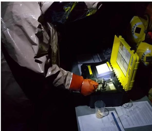
**FTIRs Must Be Usable in Various Environments and When PPE is Worn**
