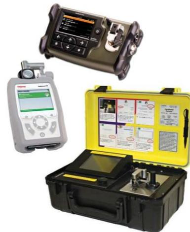
**Examples of Portable FTIR Chemical Detectors Used for Solid and Liquid Identification**
