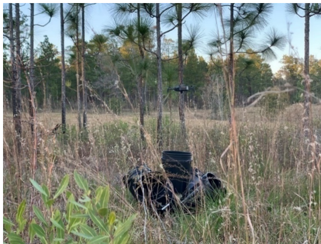
Figure 3-5 Omnidirectional Bucket Stand with Visual Acuity Targets Inside
