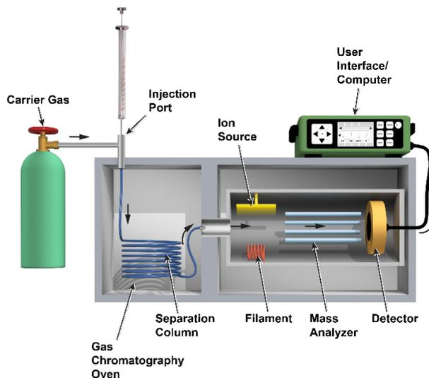
Figure 1. Schematic of a Gas Chromatography/ Mass Spectrometry System
