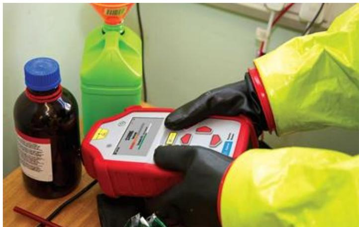
Figure 2. A user operates a handheld Raman spectrometer with heavy gloves and other PPE
