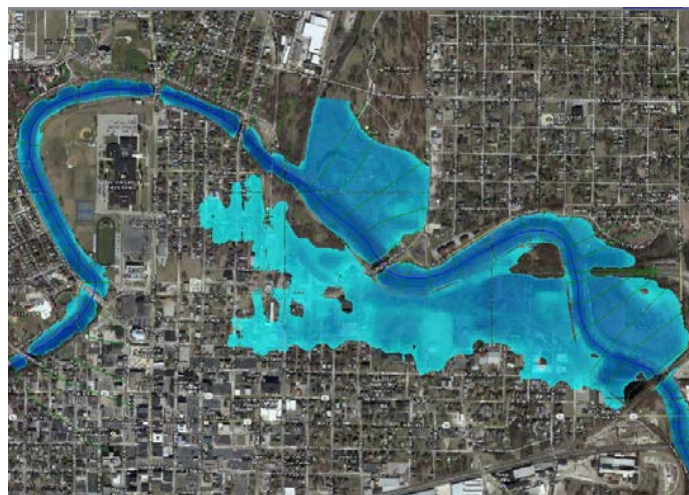
Levee break animation created by the U.S. Army Corps of Engineers Hydrologic Engineering Center's River Analysis System inundation mapping model.
