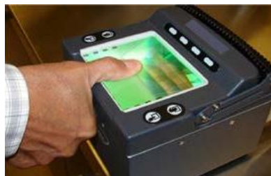
Optical scanner for electronic capture of exemplar prints. Photo courtesy of Homeland Security Investigations.
