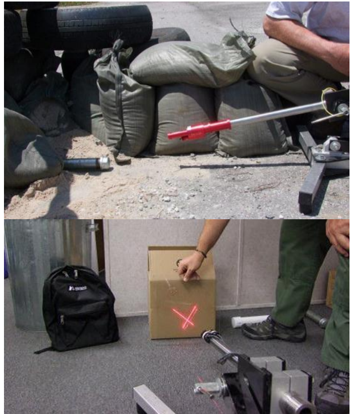
Laser aiming devices for EOD disrupters assessment.
