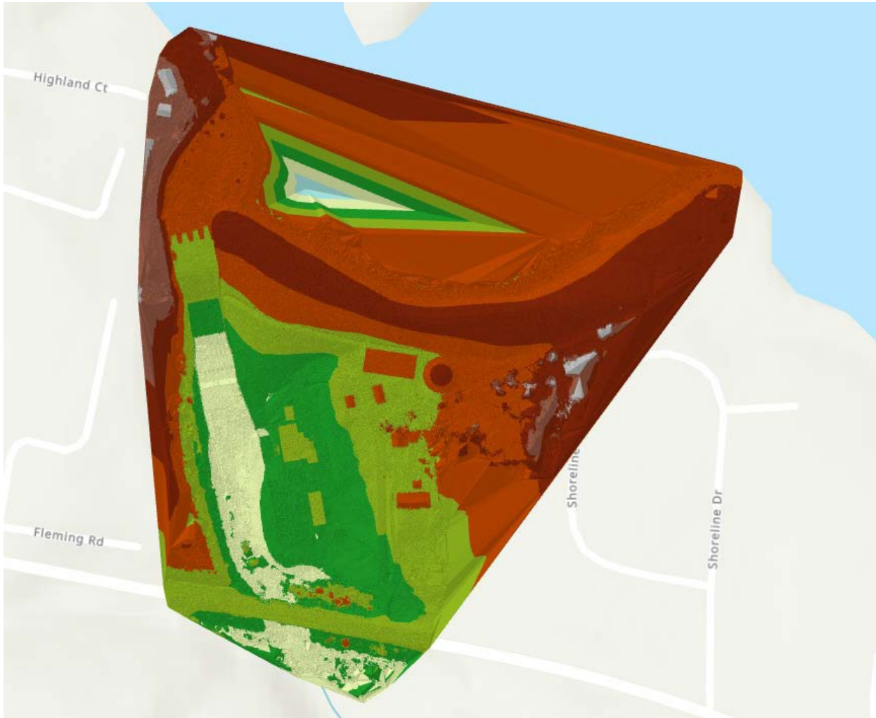
Triangulated Irregular Network (TIN) data developed from drone flight at Guist Creek Dam
