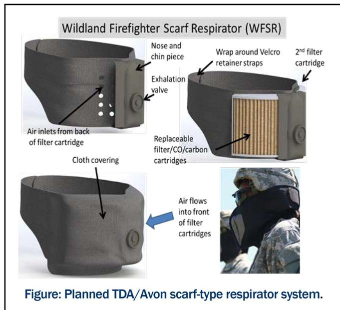
Figure: Planned TDA/Avon scarf-type respirator system.
