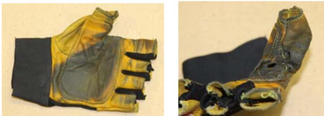
The above two photos show a used rescue hoist glove. The close up shows the intense wear area that causes a glove to fail within a short period of time.
