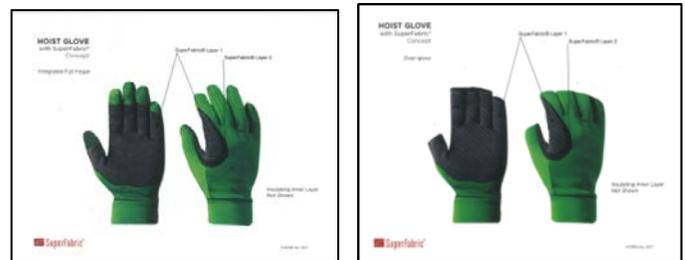
Concept drawings for the new rescue hoist glove. The drawing on the left shows the integrated concept and the drawing on the right shows the overglove concept.
