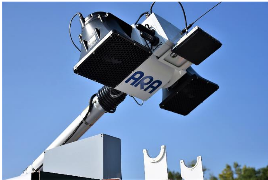
Figure 3-18 Telescopic Mast with Radar and Loudspeakers is Halfway Raised during Testing
