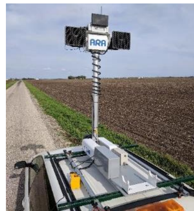
Figure 1-1 ADRAS Vehicle Mounted Deployment Courtesy of ARA
