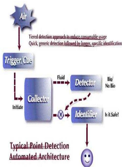
**Figure 1. Typical point detection automated architecture (with a combined trigger/cue).**
