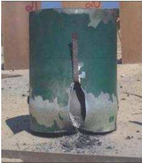
Image 2. MTR 101 breached in bottom charge location test
