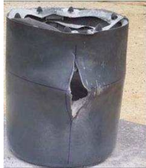
Image 3. Charge produced large hole in lidded BG40-1.6
