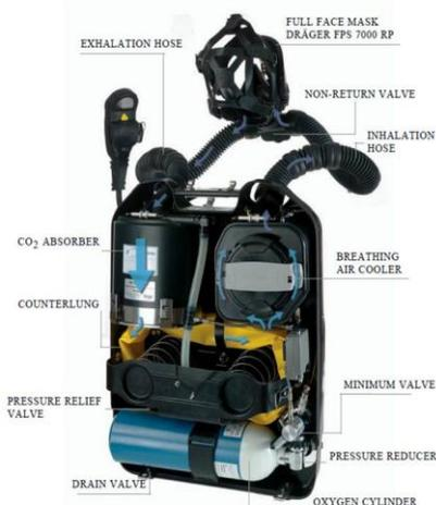
Figure 2. Loop Configuration on Dräger PSS® BG 4
