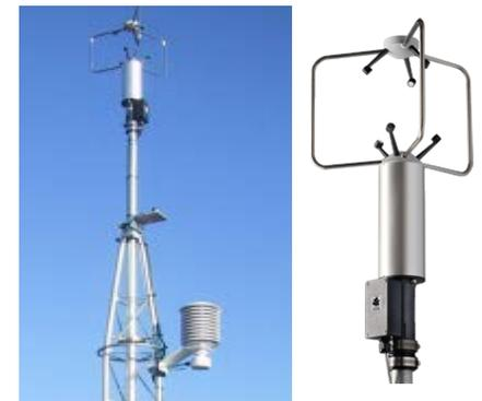
(a) Fixed Weather Station, and (b) Ultrasonic Anemometer.
