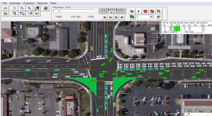
**Figure 3. SIM TRAFFIC model showing reversible lanes on street intersections**
