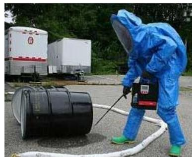
**Figure 2-2. Detecting Leaks from a Chemical Drum Using a Portable FID**
