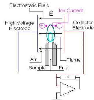
**Figure 1. Principle of Flame Ionization Detector**
