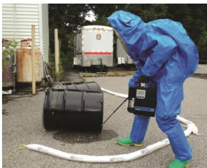
**Figure 2. Detecting Leaks from a Chemical Drum Using a Portable FID**
