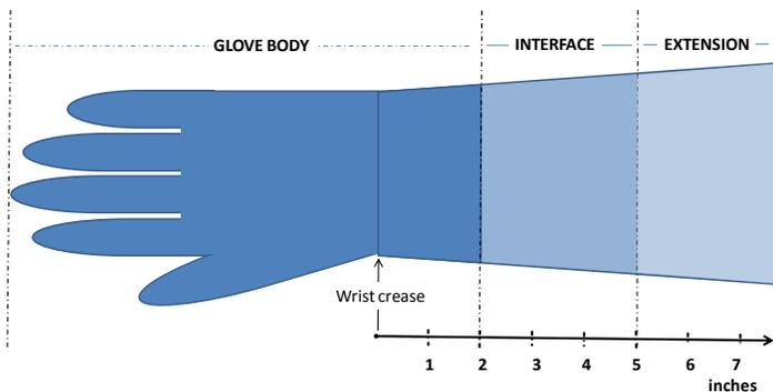
**Illustration of Glove Sections.** The distance from fingers to wrist crease is specified for standard sizing dimensions.
