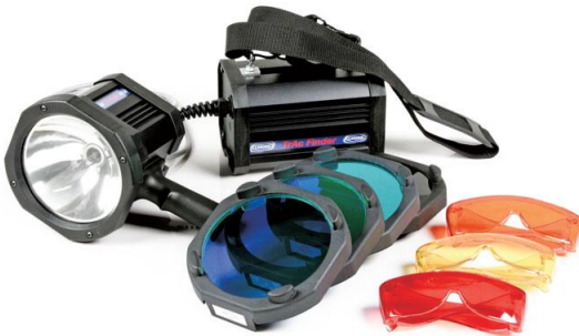
Figure 2-4. A Kit Featuring an ALS with Barrier Filters to Change the Wavelength
