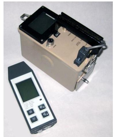
Examples of Handheld Radiation Survey Meters
