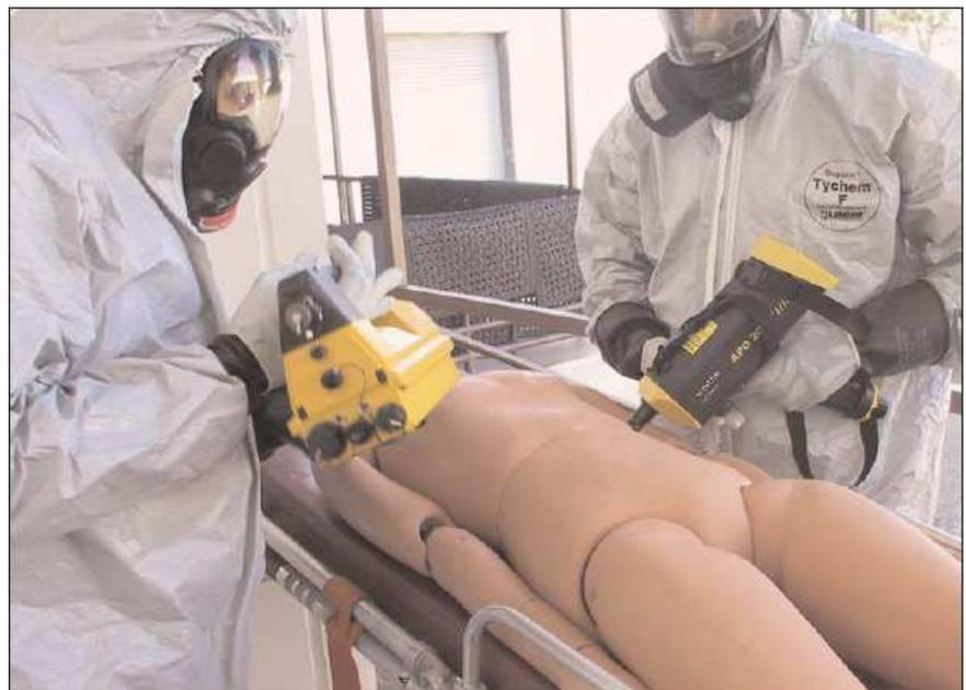
Domestic Preparedness (CDP) conducted an assessment for four IMS chemical detectors that met the Authorized Equipment List (AEL) guidelines for IMS chemical agent detectors (see table 1).
