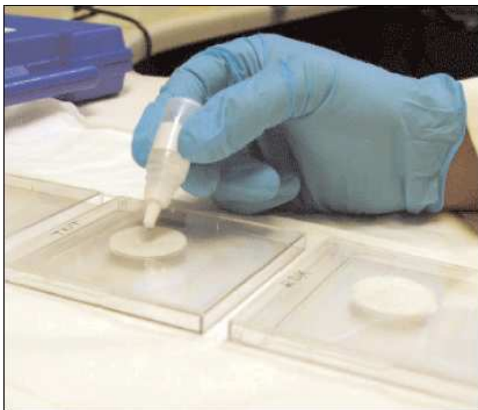
Test sample preparation. Application of single drop holding the bottle at approximately a 45 degree angle.
