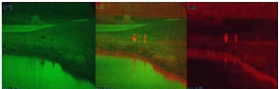
**Digital Image Fusion: Image Intensification (left), Fused Image (center), Thermal Image (right)**
