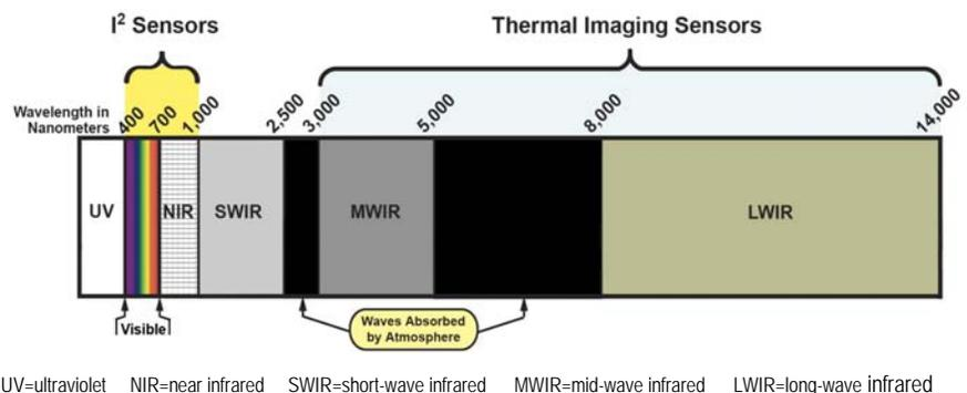
UV=ultraviolet    NIR=near infrared    SWIR=short-wave infrared    MWIR=mid-wave infrared    LWIR=long-wave infrared
