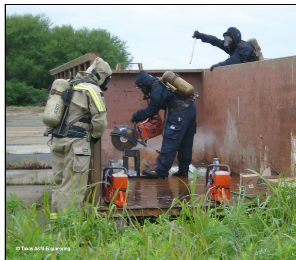
Figure 3. SMEs cut glass block as part of the multipurpose cutoff saw blade test.
