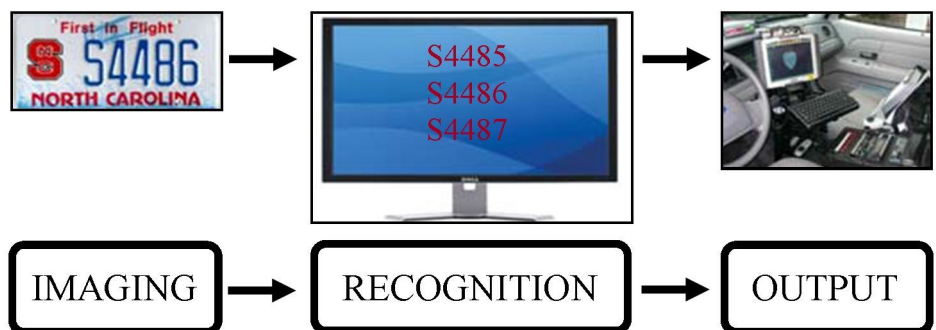
How License Plate Recognition Works
