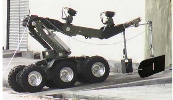
**Figure 1. Mobile x-ray system consisting of a remotely operated x-ray source and flat panel detector deployed with robotic equipment.**
