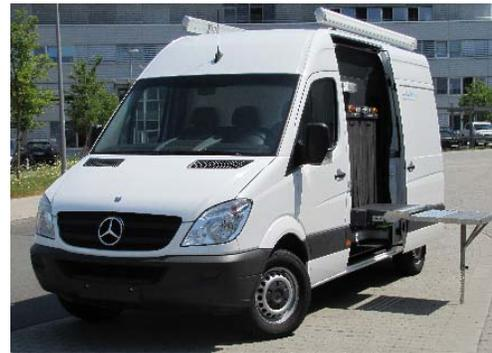
**Figure 2. Mobile x-ray system deployed in a van.**
